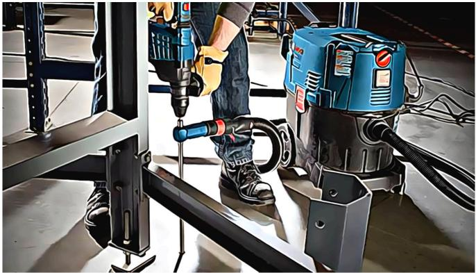
To accelerate the anchoring installation process, several manufacturers have introduced a new style of drilling bit. These <u>hollow-core bits</u> use a shaft bored down the center of the bit to draw the dust and debris directly into the vacuum while drilling. The challenge with these systems is some holes have ridges so all the debris is not extracted.
