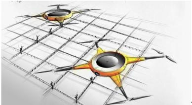
2. There are groups of inventors who are applying robotics to drone technology. For example, Skymul, an Atlanta-area startup, is developing a drone system that will tie rebar on a bridge deck. The software will control up to 8 drones equipped
